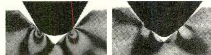
Stress analysis photos show concentrated high pressure with elliptical stylus (left), reduced pressure, less groove distortion with Shibata stylus (right).
