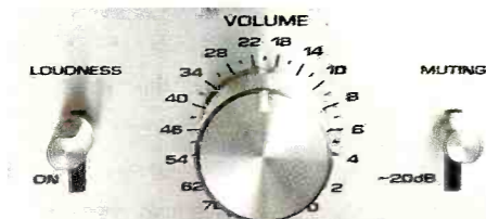
Click-stop volume control calibrated in decibels, with left/right tracking within 0.5 dB.
