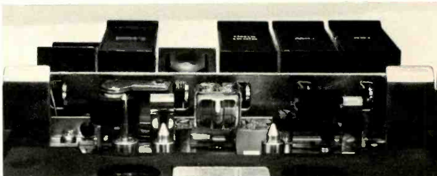
The highly refined record/playback head of the Nakamichi 500 is at center. This is the view that would be seen from the machine's rear edge, looking forward toward the transport keys.
