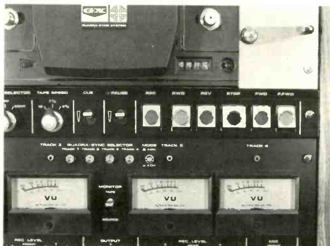
The Quadra-Sync selector buttons and mode switch are just above the four recording-level meters on the GX-400DSS.
