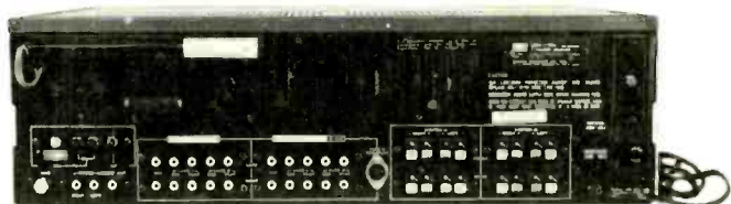
Most of the phono jacks on the 7001's rear panel are grouped arrays for the front and rear channels. The phono inputs are at lower left, while the spring-loaded speaker connectors are near the lower right.
