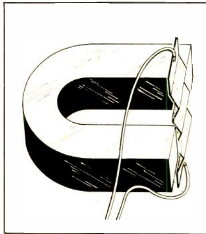
Fig. 2. The ribbon microphone is electrically identical to the moving-coil design, but the moving mass is lower because of the lighter diaphragm and the absence of a coil. Unmodified ribbon microphones exhibit a bidirectional pickup pattern.
