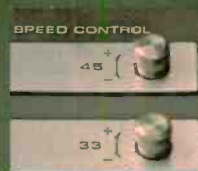
Electronic speed adjustment for each speed.
