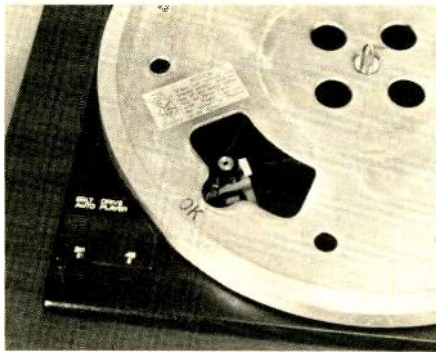
The drive pulley of the Hitachi PS-12 is accessible through a cut-out in the platter. This permits easy belt removal and replacement.
