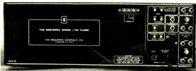
Among the features of the Model 1's rear panel are controls for the oscilloscope (focus, intensity, position), means of selecting the amount of de-emphasis, and scope inputs for external signal sources.
