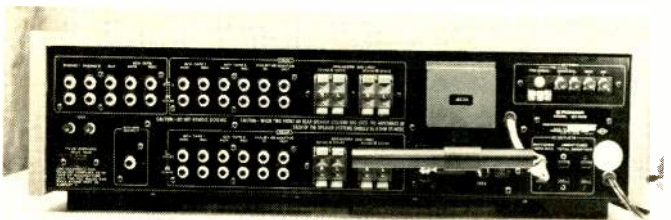
All the connectors for front-channel sources and speakers are arrayed along the top half of the 949's rear panel, with rear-channel connectors directly below. Two-channel sources plug in at upper left.
