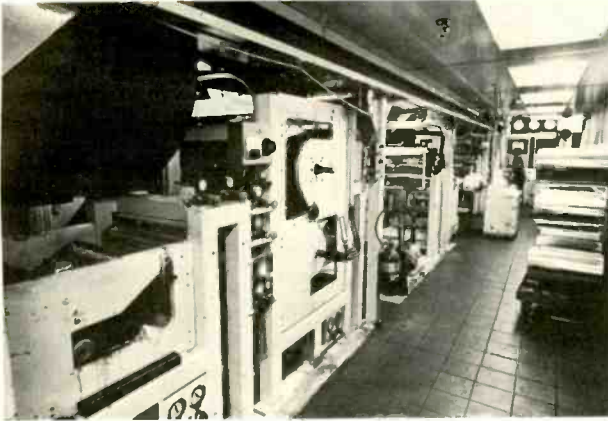
Above is but a small part of one of the giant coating machines: in this section the film is fed into the machine, coated, and exposed to a magnetic field to orient the iron-oxide particles.
