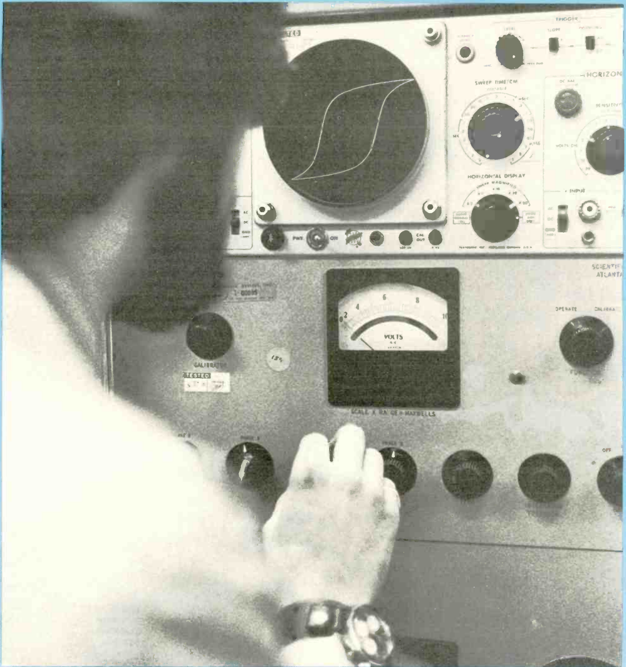
The hysteresis loop displayed on the oscilloscope simultaneously shows the magnetic force needed to magnetize a given tape as well as the amount of magnetism it will retain once magnetized. These properties are important indicators of tape performance.
