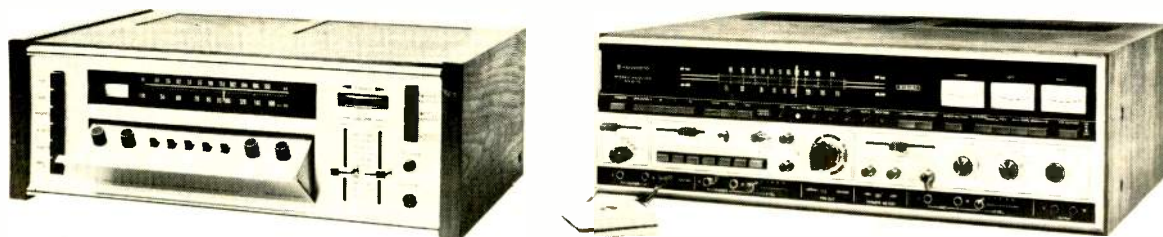
The distinguishing features of many new receivers are "up front" where they can be seen. The four-channel Dokorder MR-800Q has a novel flip-down control panel. The Kenwood KR-6170 has only two channels, but keeps both very busy.
