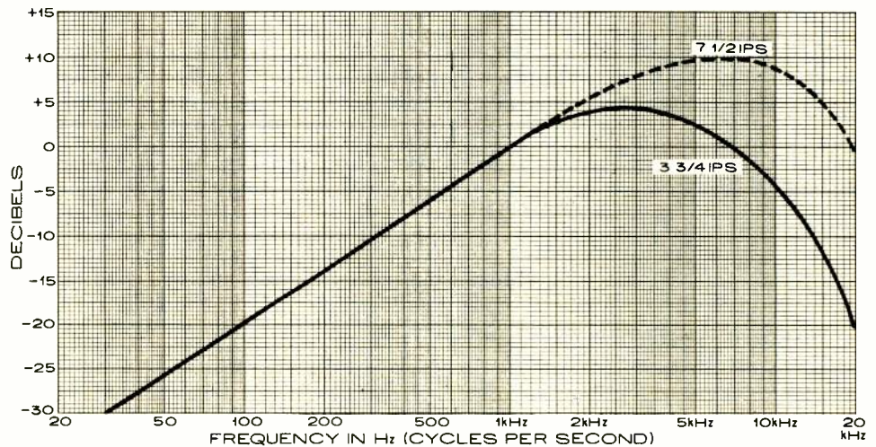
Fig. 1. An unequalized playback head's response to equal-strength taped audio signals of various frequencies. The 6-dB-per-octave rise with frequency continues until the recorded wavelengths for the two tape speeds begin to approach the width of the head gap.
