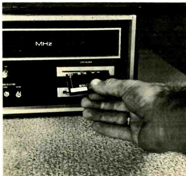
The plug-in programming card inserts into a front-panel slot below and to the right of the digital-readout tuning indicator. A prepunched card is provided for each of the 100 FM channels.
