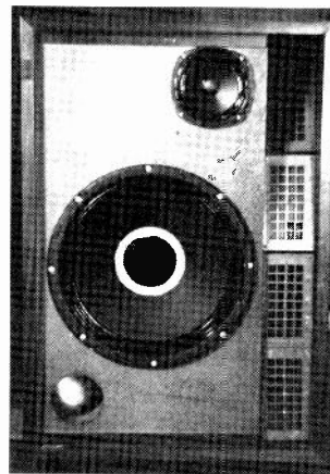
The Infinity 2000A speaker system employs four electrostatic elements, two of them pointed slightly upwards. The enclosure's port is visible at the lower left corner.
