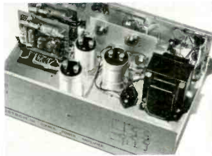
Step 1. Kit is designed so you can stop after wiring the easy-to-assemble power-amplifier stages, if you already own a hi-fi preamplifier. Construction time: about five hours.
