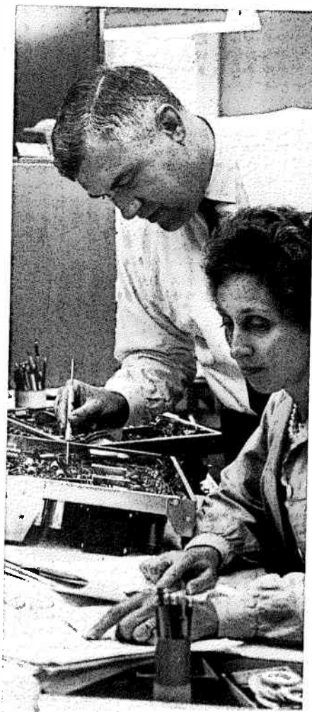
Gaylord Russell overseeing kit construction. Here, a kit is being built to a "rough draft" instruction book. Before any kit is shipped from the plant, about 50 pre-production kits are built in order to assure accuracy of the instruction book.
