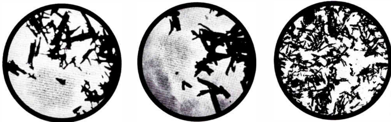
Flaws in the oxide coating are not usually visible to the naked eye. Photomicrographs, however, reveal such problems as uneven oxide-particle dispersion (shown above), which causes hiss and noise, and also high-frequency losses in recording and playback.
