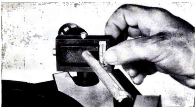
stylus force applied directly at pivot, preserving perfect mass balance of tonearm
