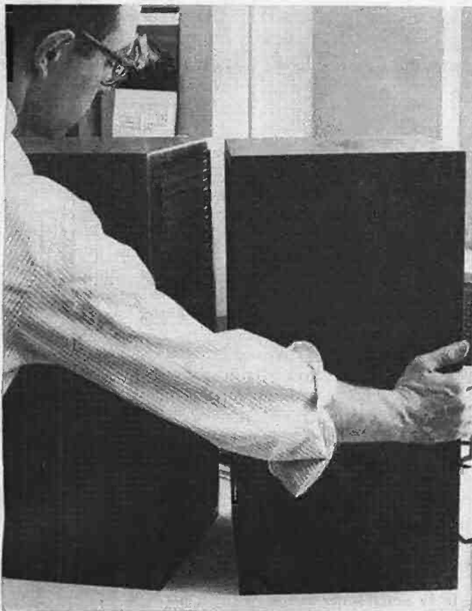
Face to face, two speakers burble bass at each other. If they are connected out-of-phase, the lows deteriorate due to mutual cancellation. This arrangement makes a quick "ear test" for phasing.
