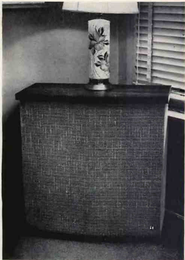
LATEST TRUSONIC SPEAKER SYSTEM from Stephens uses a bass-reflex ducted-port enclosure. Our reviewers found it to be exceptionally "easy to listen to." The speaker was a 15-inch coaxial Stephens Model 150CX.
