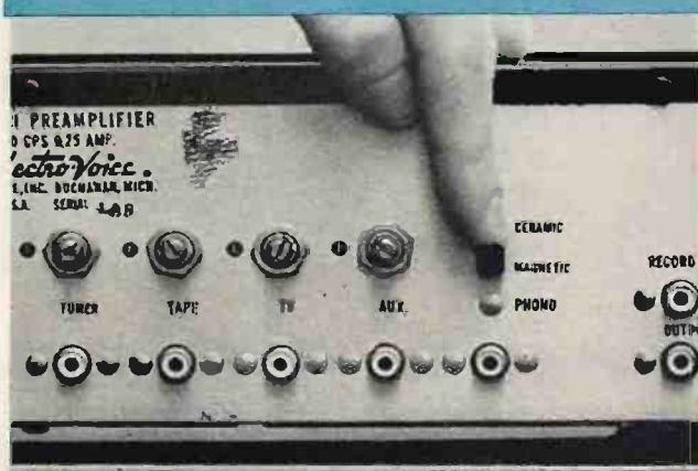
Controls behind the scenes sometimes include a switch for choosing between ceramic (or crystal) and magnetic phono cartridges.
