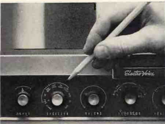
The Electro-Voice selector knob chooses the record compensation when the signal source is a phono record.
