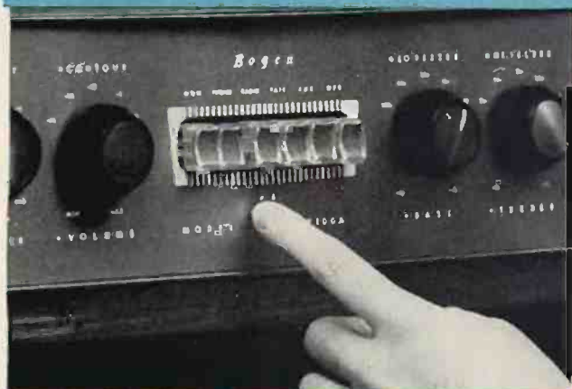
Bogen supplies a front panel switch for choosing between two turntables or a turntable and a changer, both with magnetic cartridges.
