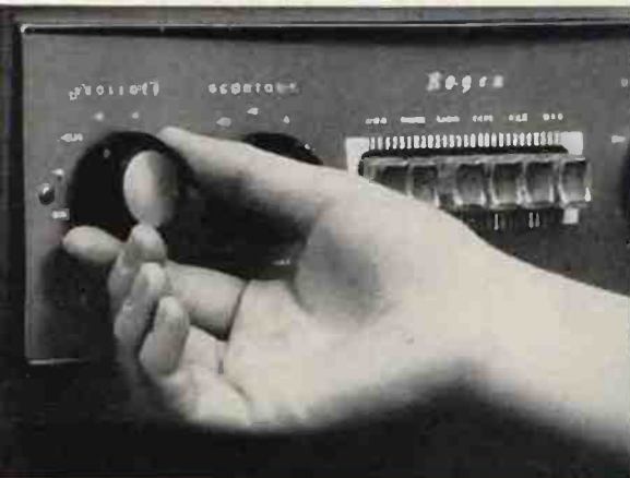
Bogen uses two knobs, one within the other, for record compensation: one for treble rolloff, the other for bass turnover.
