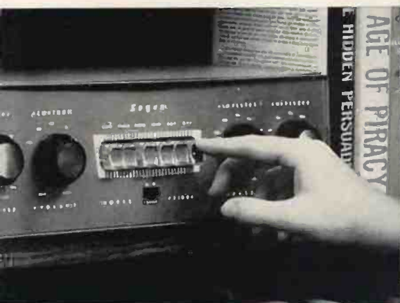
The Bogen function selector consists of a series of push buttons that route the signal from its source to the amplifier.
