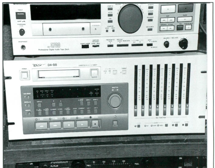
Figure 1. One of the six Tascam DA-88s that are located in the truck. Linked together these provide 48 tracks of digital audio.
