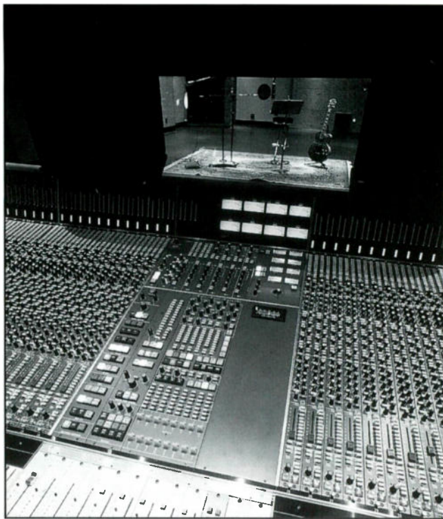
Figure 8. A close-up view of the Neve Legend's center area. A VSP Section handles complex speaker configurations for film mixing
