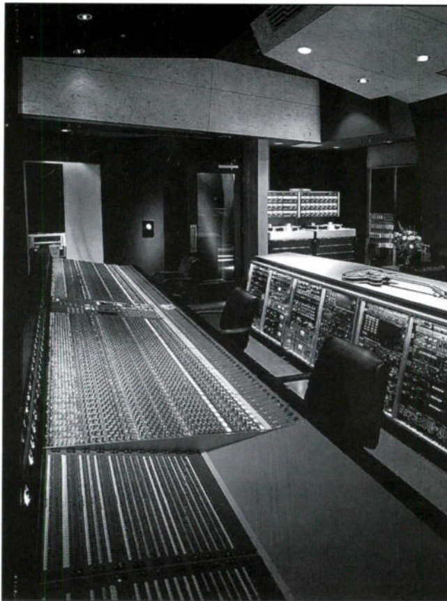
Figure 1. Pride of the place in the new SSL 1 Studio Suite is this 96-input SL-8000G.
