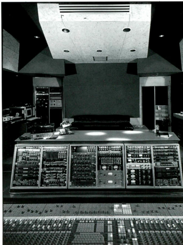
Figure 3. A view from the front of SSL I. It shows the well-equipped outboard rack situated behind the engineer's mix position.
