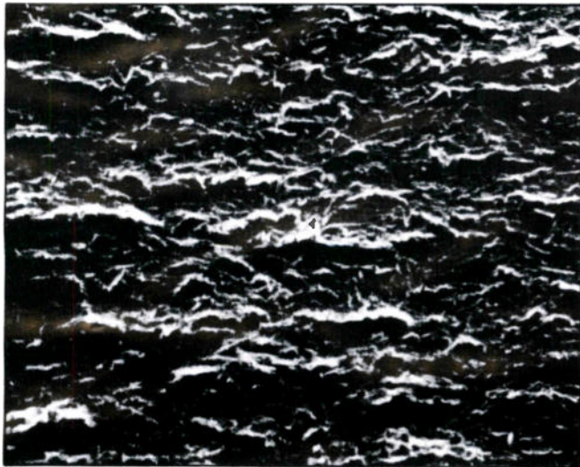
Figure 2. These electron scanning microscope photographs, processed at a diameter magnification of 10,000 and a viewing angle of 45 degrees to the surface, show differences between the Ampex 456 analog (left) and the Ampex 466 high-energy digital tapes. At this magnification, the surface roughness is directly related to the gloss level under standard viewing—the lower the surface porosity, the higher the gloss, as seen in the 466 photograph on the right.
