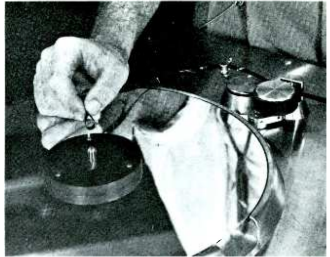
Threading the 14"-diameter open-faced "reel." Reel held 5400 ft. 0.002" thick tape. Torque/threading pin mounting circle dimensions have carried over to present day N.A.B. Standard Hubs as inside (hub bore) driving slots.
