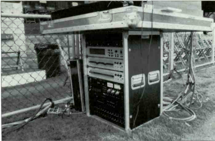
Figure 4. The mix console sits on one of two portable equalization, playback, and amplification racks.
