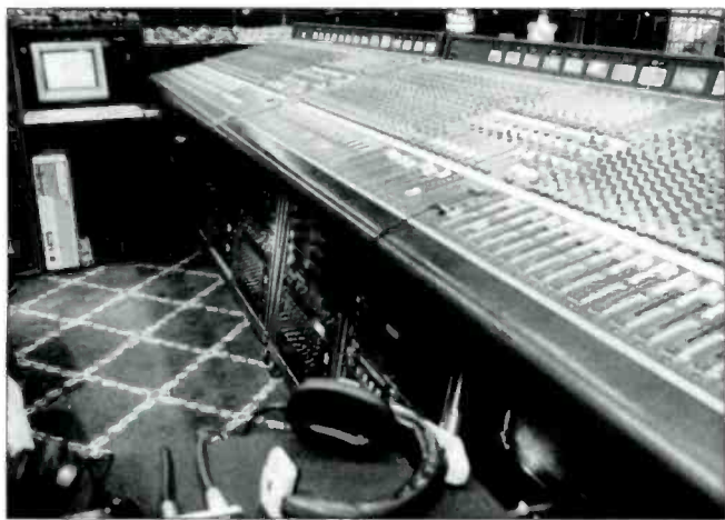
Figure 2. A closer view of the house sound booth showing the effects racks below the console and, at top left, the control computer.
