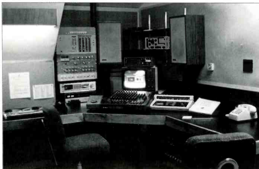
Figure 18. The mixing position. Note the SMPTE controls surrounding the console, and a spectrum analyser sitting atop the video monitor.
