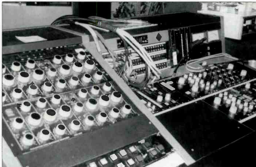
Figure 4. The modified Neumann Analog Mastering Console. The row of knobs at left are part of a Sontec Mastering EQ.
