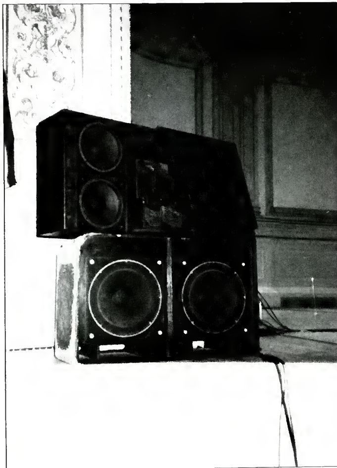
Figure 3. The house sound system for Judy Collins and Arlo Guthrie's performances at Carnegie Hall. Note that the left hand mid-high cabinet wears lenses to increase dispersion of the high and super-high horns, while the right-hand box has been tilted at a 30° angle to cover the balconies.
