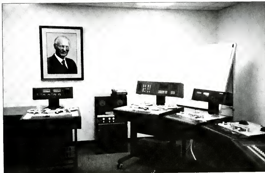
Figure 3. A procession of Studer's recording technology tape decks. From left to right, Studer A-820 two-track, ReVox B77, DASH format digital machine, A-807, A-807 rack mountable, and a corner of a 900 series console. Founder and chief executive, Willi Studer's portrait hangs on the wall.
