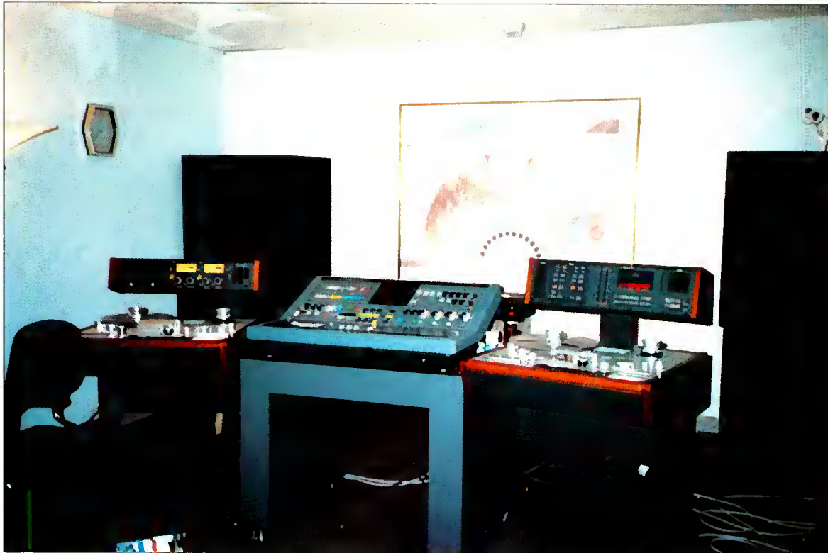
Figure 1. The digital mastering suite. At left, a Studer A-820, the Studer DASH at right, and the Neve DTC-1 console at center.
