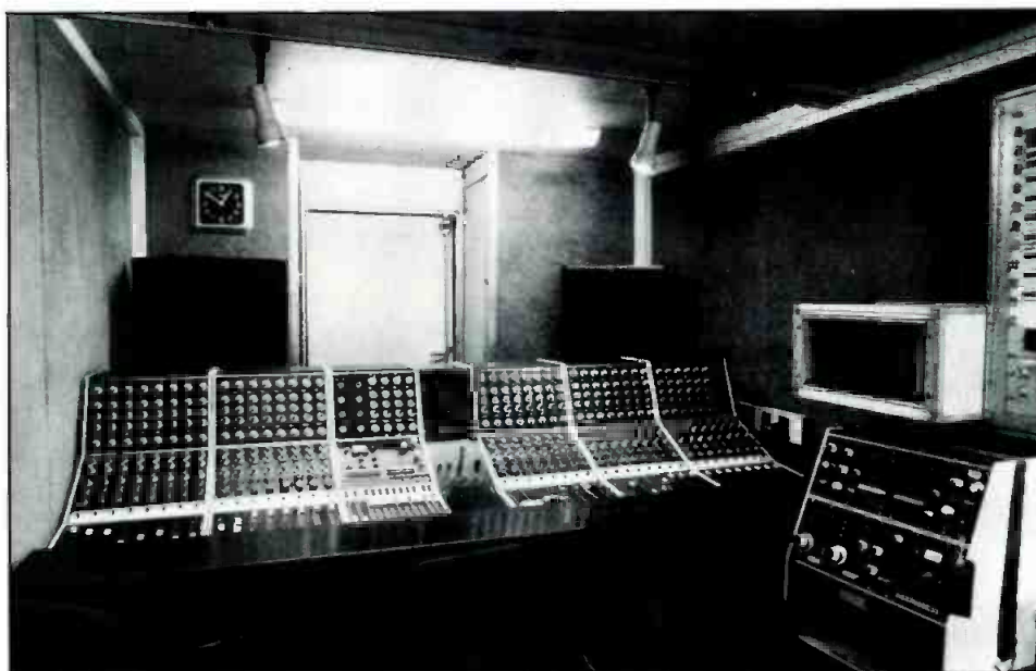
Figure 4. Interior of Type B stereo control vehicle featuring a 40-channel Calrec mixer.
