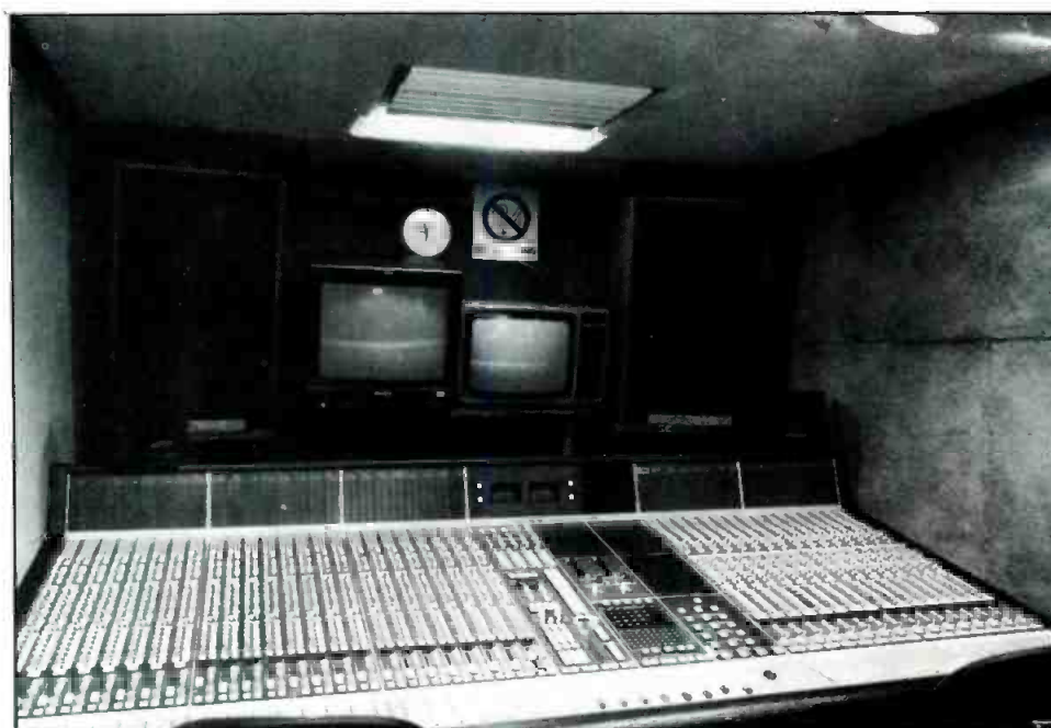
Figure 1. Interior of Type A stereo control vehicle featuring 40-channel solid state logic console.
