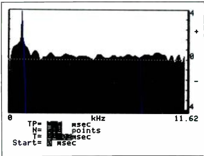
Figure 8. Group delay plot of system (measured in msec) as tuned by the third-octave equalizer.
