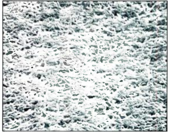
Figure 2. These electron scanning microscope photographs, processed at a diameter magnification of 10,000 and a viewing angle of 45 degrees to the surface, show differences between the Ampex 456 analog (left) and the Ampex 466 high-energy digital tapes. At this magnification, the surface roughness is directly related to the gloss level under standard viewing—the lower the surface porosity, the higher the gloss, as seen in the 466 photograph on the right.
