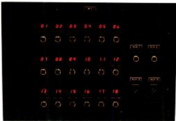
Patchable microphone input panel with digital display of console I/O assignment.
