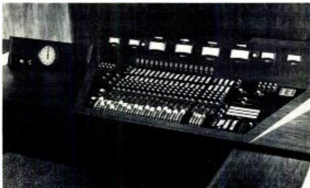
Criteria's first custom-made 4-track console designed for Criteria by Jeep Harned of MCI.
