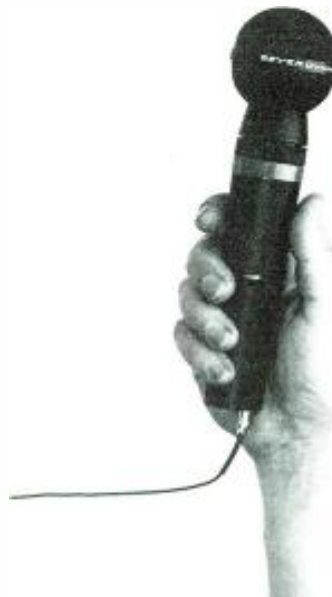
Figure 6. Beyer's SM 85 is a universal radio microphone transmitter, which will accept a variety of plug-in microphone capsules.
