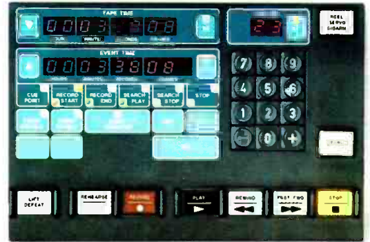
ATR-124's Multi-Point Search-To-Cue (MPSTC). Provides 100 cue locations.
