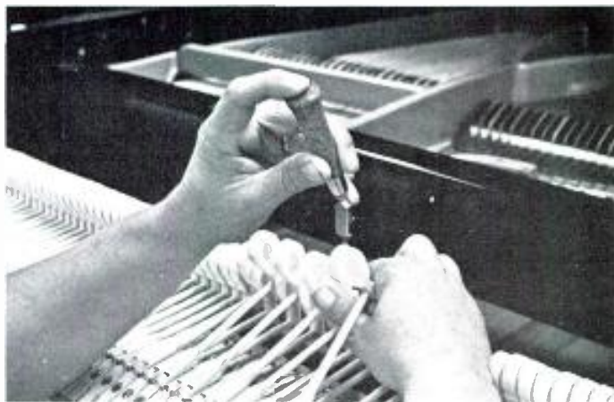
Figure 5. A close-up of the voicing process, best handled by a skilled piano technician.
