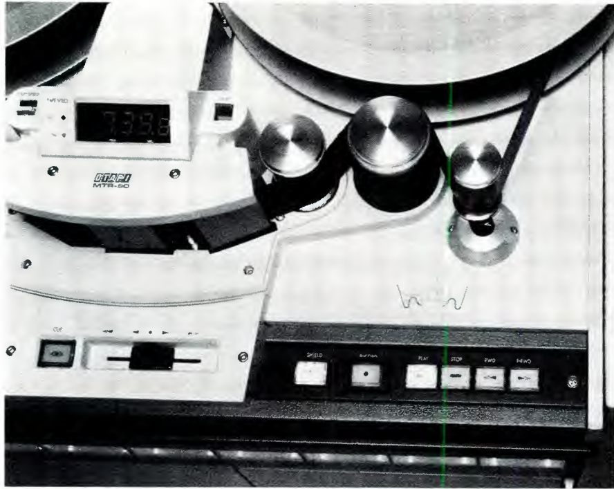
Figure 2. Note that the servo capstan drives the back coating side of the tape, minimizing slippage and oxide abrasion.
