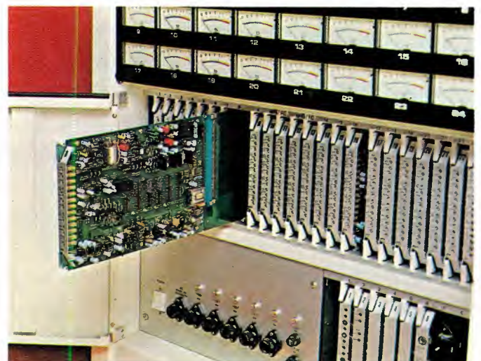
Figure 4. A single plug-in card for each track contains record, sync and repro electronics. At the bottom is the power supply, and plug-in cards for the transport servo, master bias and test input patch point.
