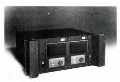
• The Model 6500 amplifier offers modular construction which allows the user to remove either channel for inspection or exchange while the amplifier is mounted in the rack. Each channel is totally independent with its own power supply and even its own continuously variable cooling fan. The Model 6500 provides 275 watts RMS at 8 ohms with .1 percent THD and up to 1,200 watts RMS in mono mode at 4 ohms.
