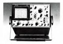
• The V-550B oscilloscope offers a 6-inch square CRT with an internal graticule. The use of an improved metal backed phosphor makes the 10 kV tube as bright as the older 15 kV CRT. Among the features are: trigger view, variable trigger hold-off, full TV triggering and single sweep capability. An additional feature is automatic focus correction which restores proper focus whenever intensity or sweep range control settings are altered.
