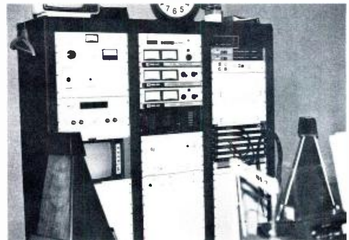
Figure 9. The control room equipment rack. Note the dbx and Dolby noise reduction systems, as well as the Sequerra tuner.
