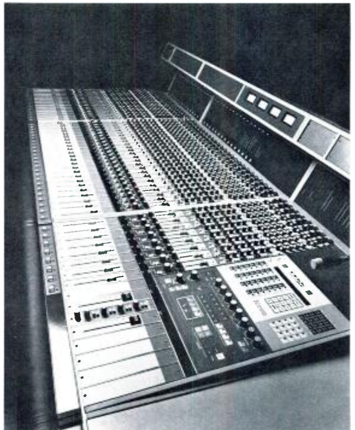
The Neve 8108 Series recording console. Note assignment panels in foreground, and barograph meters along the raised panel.
