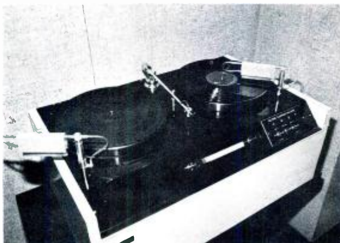
Figure 8. Each record is cleaned, prior to being aired, on the Keith Monks Record Cleaning Machine.
