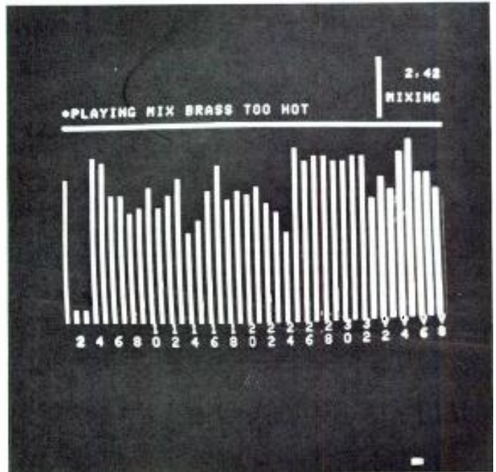
Figure 5. The bar graph shows the d.c. levels generated by each fader.
