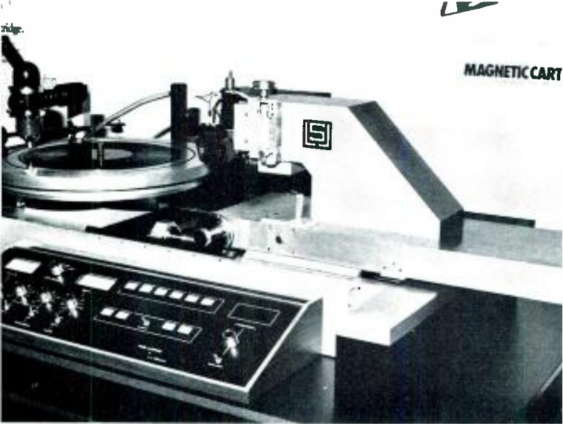
Larry J. Scully is making this advanced disc recording lathe and selling it in the U.S. in conjunction with Ortofon heads and electronics.
