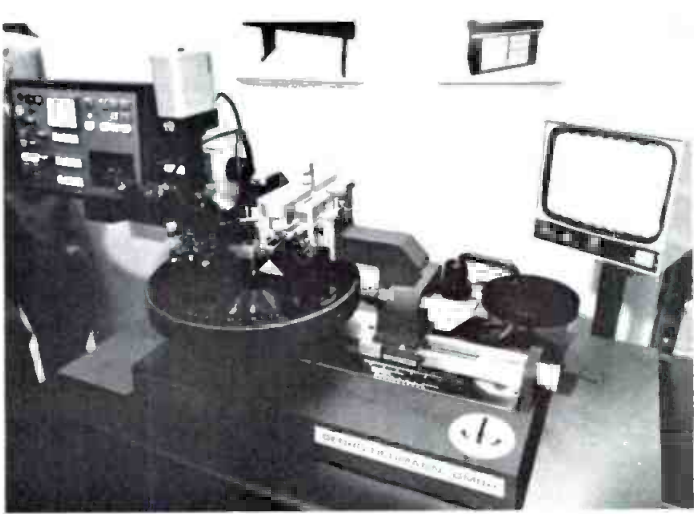
The Neumann VMS 80 disc mastering system. Note the video camera on it, and also note the adjoining crt display.
