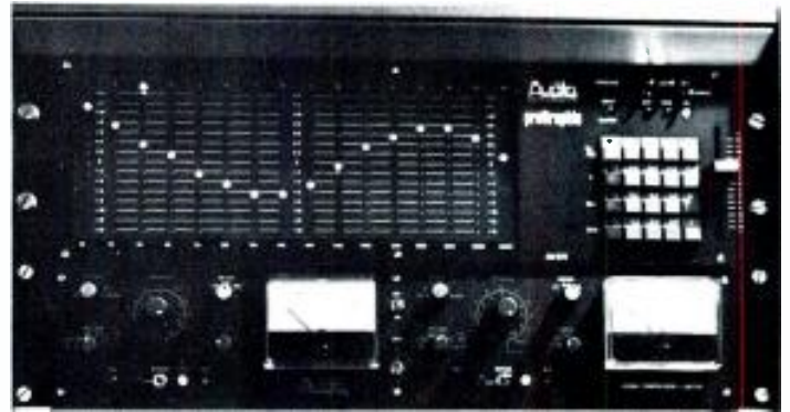
Audio Developments' proGraphic Equalizer. You can also see the AD 055 Compressor/Limiter just below it.
