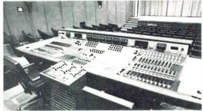
The Ward Beck console at the National Film Board of Canada can handle up to 96 tracks with its pre-mix sub system.
