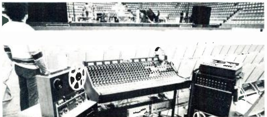
Gene Clair (left) setting up for the Elton John concert at the Forum. Their custom console (foreground) takes 30 channels mixed to a 4-way system.
