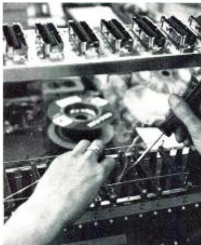
A bird's eye view of the WKRC card files being mounted in their rack.
