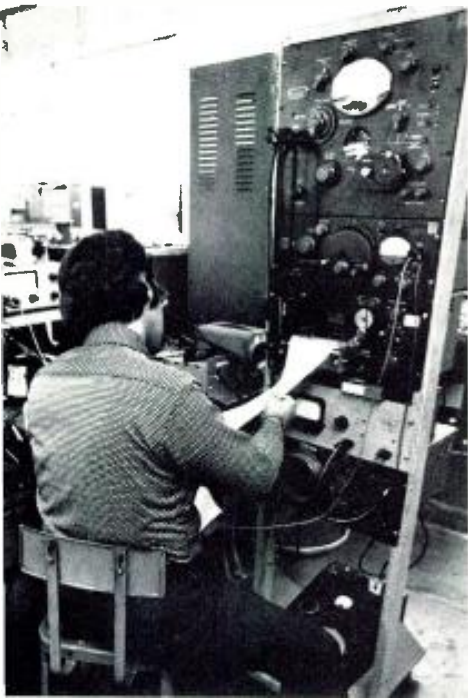
The engineering lab uses an automatic frequency spectrum analyzer to check out prototypes.
