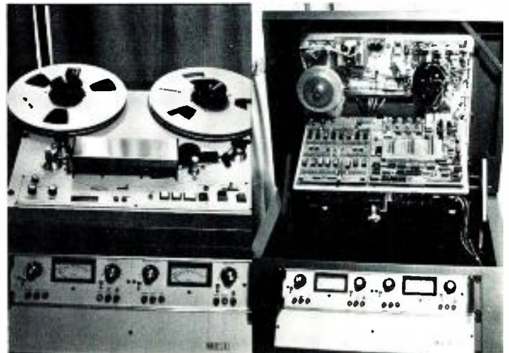
MCI's series JH-110 tape recorder. At right the transport is raised to show its undersides.
