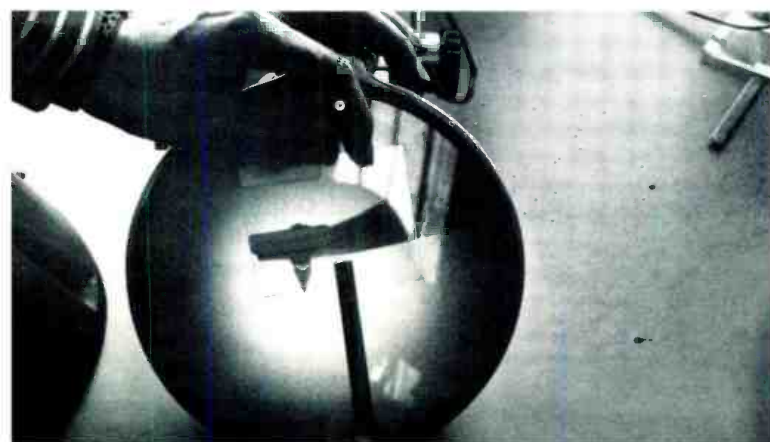
The shadow spectrograph is a useful tool in many areas of Ortofon's production. Here it is being used as a proof of correctness check on the stylus assembly of phono cartridge.
