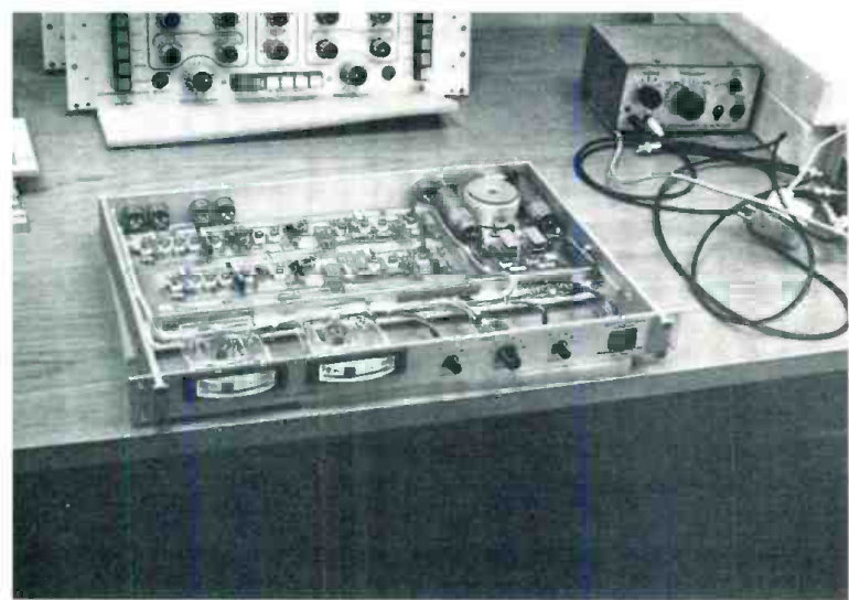
Another corner of the lab is used for the assembly of electronic components such as this finished regulated filter here undergoing tests.
