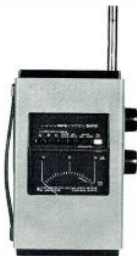
Figure 1. A precision sound level meter such as this is required for room analysis.
