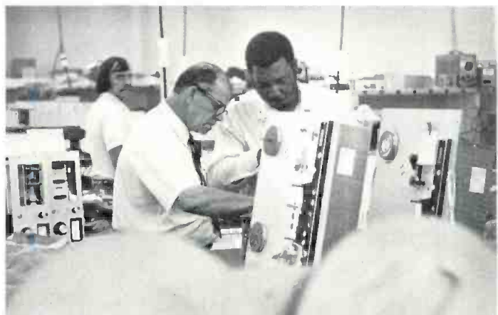
A partly finished Scully 280 takes shape under the hands of Willie Pittman (right) and Ray Reynolds.
