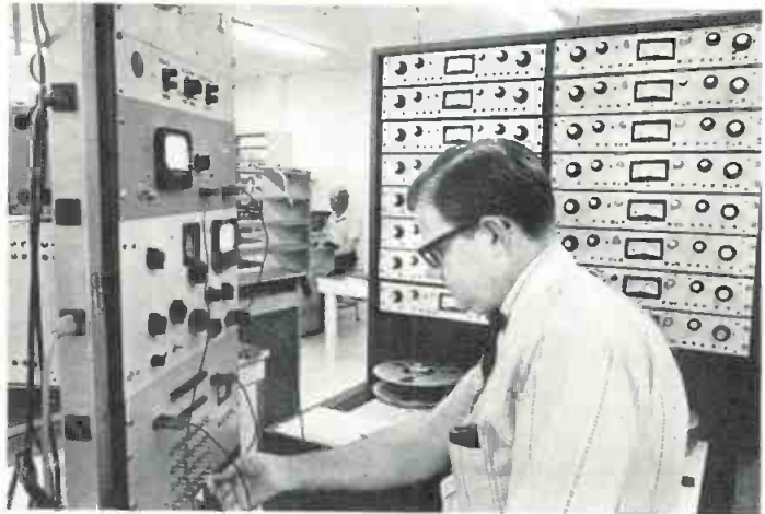
When the line work is finished, a Scully 280 goes to an individual calibration station.
