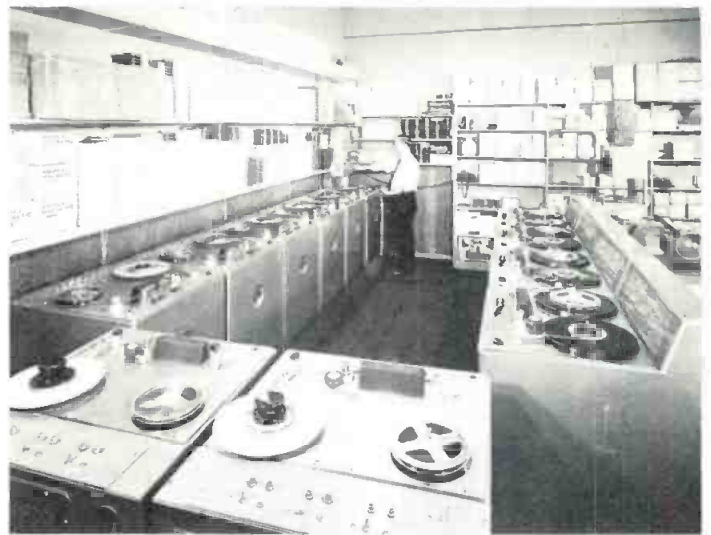
Figure 3. Twelve open reel Ampex slaves can turn out a lot of per-hour copies. Not shown are the master machine and the Pentagon cassette duplicating equipment, also located in this room.
