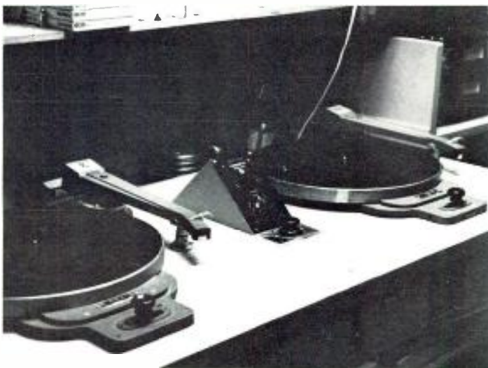
Figure 4. Two Rek-O-Kut turntables and a central switcher serve for disc dubbing and audition.
