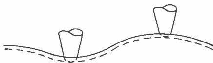
Figure 3. The same stylus as in Figure 2. This time it is tracing a long wavelength.
