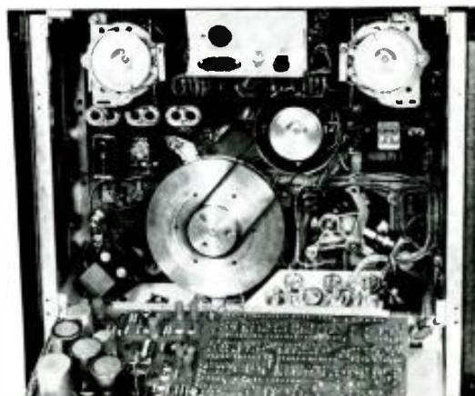
Figure 11. Front and rear views of the Philips PRO 36 transport utilizing the capstan drive described in this article.
