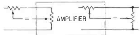
Figure 1. The theoretical conditions required for voltage gain and insertion gain to have the same significance, relative to an amplifier.
