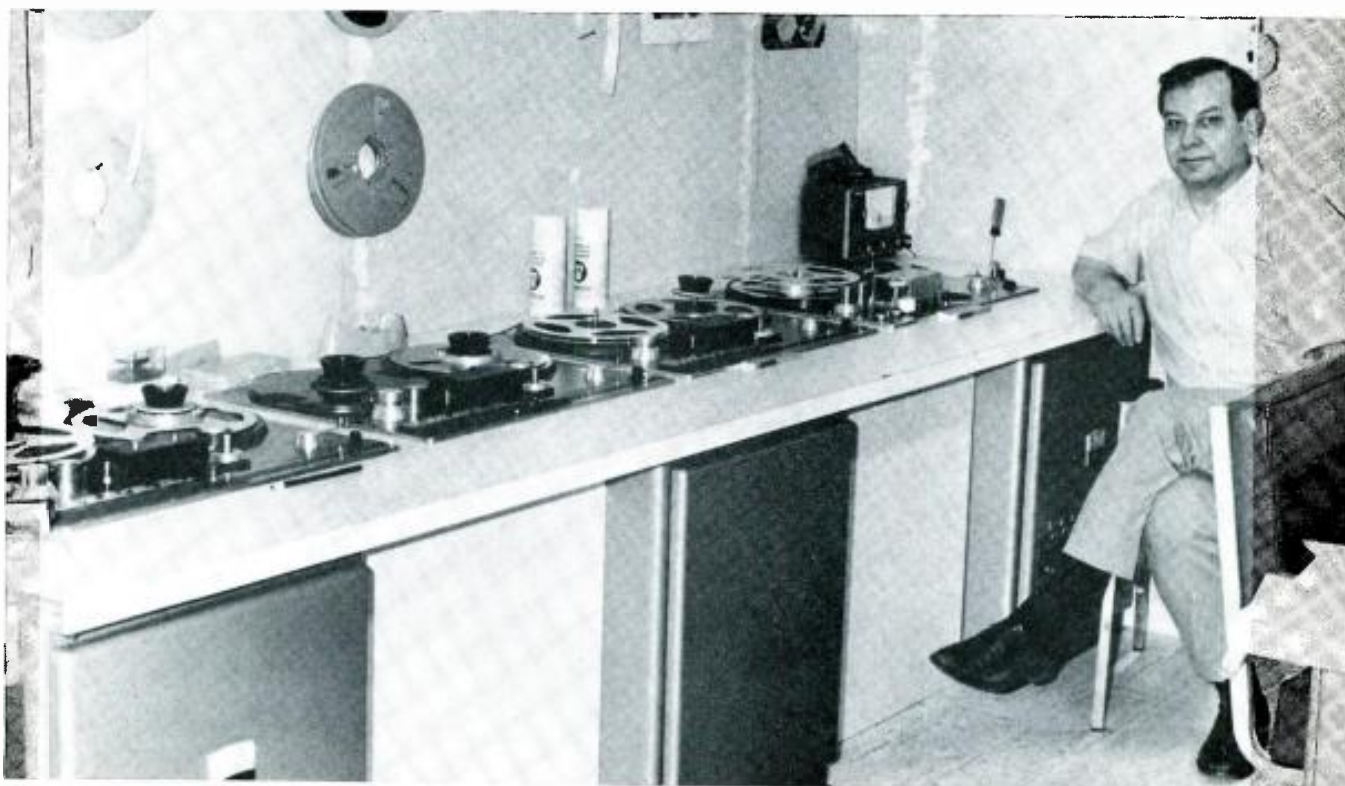
Figure 2. The tape-deck console. Each of the three pedestals has a bias-erase generator amplifier, eight f.e.t. reproduce preamps, and the
