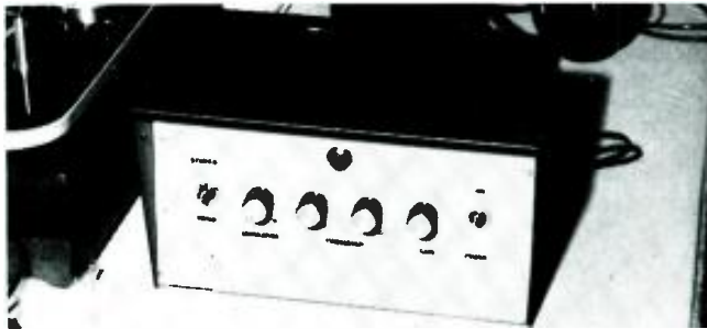
Orban Associates (R.A. Moog). Stereo Synthesizer. Creates a distortion-free stereo synthesis offering maximum fidelity to the mono source. The unit shown is a prototype. Production units will look slightly different. Price: $895. Circle 93 on Reader Service Card.
