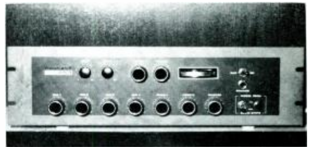
Harman-Kardon Inc. ProcasT 5600 mixer/preamplifier. Output +18 dBm, less than 0.25 per cent distortion, -125 dBm noise. Price: $310.00. Circle 95 on Reader Service Card.
