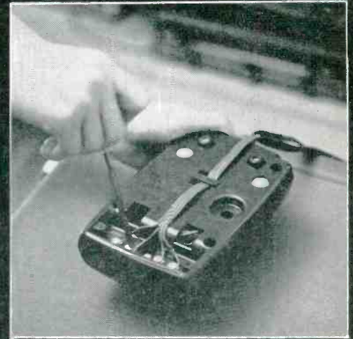
22 Rotator wires are attached to control box and antenna is ready to operate.
