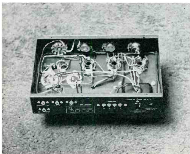
Figs. 1 and 2. Here is the Grommes LJ-6K control amplifier at an early stage of construction. Filament and power-supply wiring has been completed; sockets and controls are installed.
