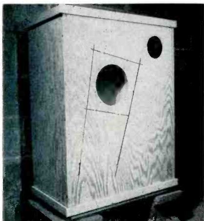
Front panel comes with lines scribed for screws or nails to hold cavity assembly.
