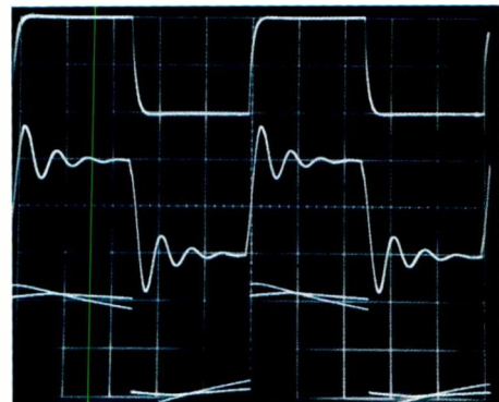
Fig. 2—Square-wave response for 10 kHz into 8 ohms (top), 10 kHz into 8 ohms paralleled by 2 μF (middle), and 40 Hz into 8 ohms (bottom). The overlaid 40-Hz traces represent response at two different output levels, with the one showing the flatter top scaled at the same 5 volts per vertical division as the 10-kHz traces and the other scaled at 1 volt per division (see text).
