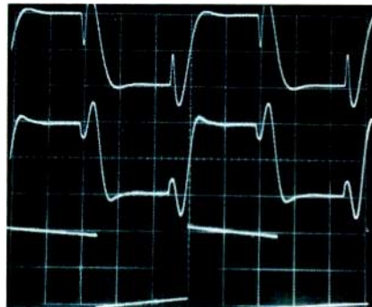
Fig. 2—Square-wave response for 5 kHz into 8 ohms (top), 5 kHz into 8 ohms paralleled by 2 \mu F (middle), and 40 Hz into 8 ohms (bottom).
