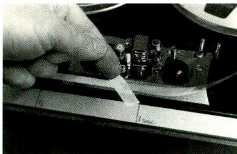
FIG. 7—REBURNISHING, ON A NONMAGNETIC SURFACE
