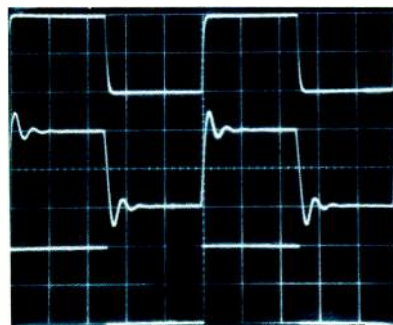
Fig. 2—Square-wave response of (from top) 10 kHz, 8 ohms (20 \mu S/div.); 10 kHz, 8 ohms & 2 \mu F (20 \mu S/div.); 40 Hz, 8 ohms (5 mS/div.); all 5 V/div. on vertical scale).
