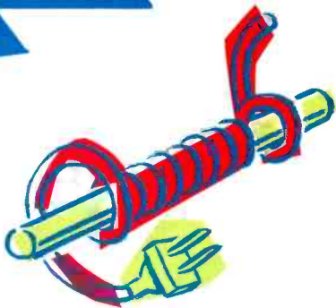
Another filter type: A power or signal lead wrapped around the ferrite core from an old AM antenna.
